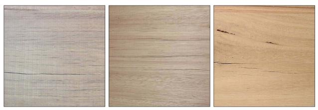
Checks are a separation of the wood fibre and differ from a split in that they do not travel from one surface of a board to another. They can often occur with rapid drying and be over much of the board surface. However, grain
